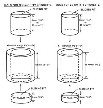
Note 1—Material: cold rolled or stainless steel. Dimensions a and b (inside diameters) are nominally 32 and 25 mm. If an automatic polishing attachment is to be used, these dimensions should be specified to yield a briquette fitting snugly in the briquette holder.
